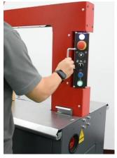
**#Turnable control panel (0°~180°)** so you don't have to turn the machine around every time when you're operating on the other side.
