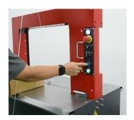
After removing strap push reset button again to close strap arch
