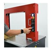
Push the Reset Button to open strap arch.
